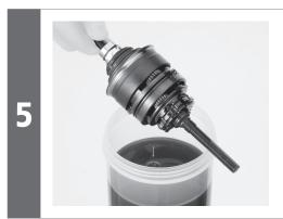
Let the excess oil drain off for approximately 60 seconds.
