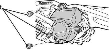
**4.** Remove the cam unit and the chain stabilizer.
