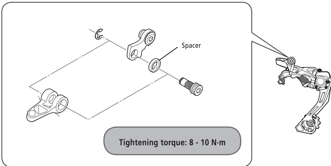
When replacing the direct mount type with the bracket-equipped type, reverse the procedure.
