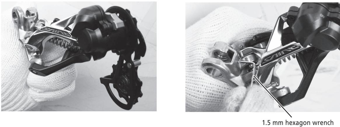
6. Remove the bump stopper holder with a narrow-tipped tool.
