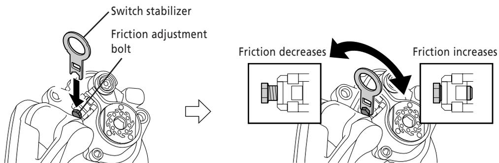
**5.** Check the friction torque.
