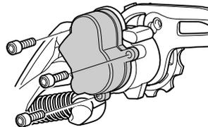
4. Remove the switch stabilizer and the chain stabilizer.
