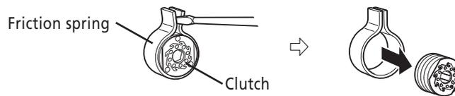
3. Apply grease to the clutch.
