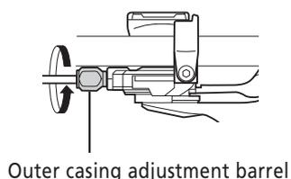
Outer casing adjustment barrel
