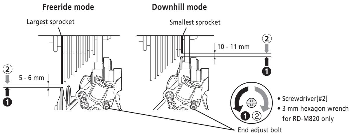
3. If the frame interferes with the rear derailleur on models with a bump stopper when the plate unit is lifted up, turn the end adjust bolt until there is no interference.
