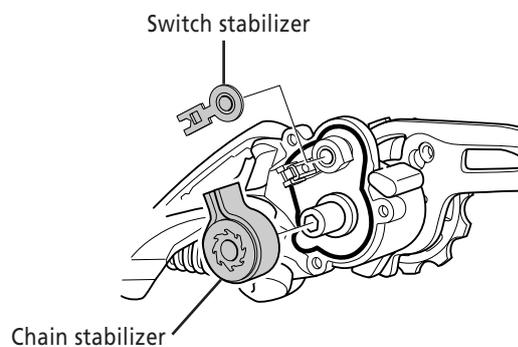
5. Use a 4 mm hexagon wrench to remove the plate axle.
