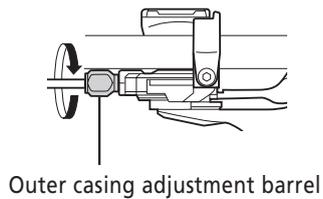
Outer casing adjustment barrel
