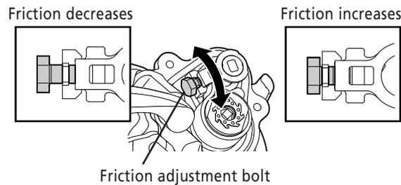
4. Check the friction torque.
