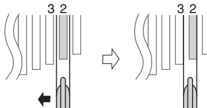
4. Return the lever to its original position (the position where the lever is at the 2nd sprocket setting and it has been released) and then turn the crank arm clockwise.
