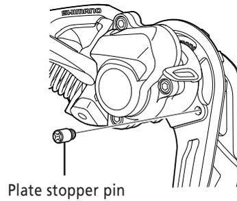
2. Turn the plate to loosen the plate tension spring as shown in the illustration.
