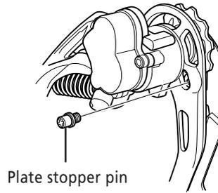
2. Turn the plate to loosen the plate tension spring as shown in the illustration.
