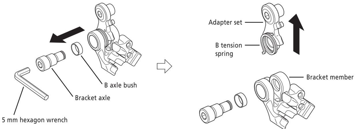
**Tightening torque: 8 - 10 N·m**
